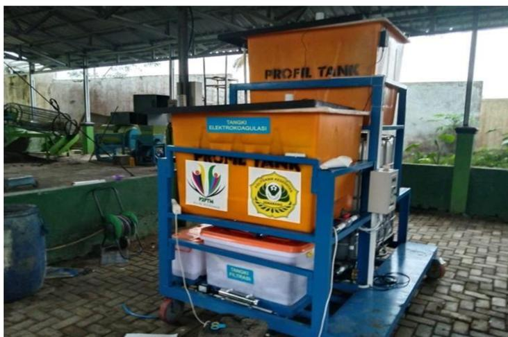
**Figure 1.** Peat water treatment equipment into drinking water with electrocoagulation system, double media filtration and UV light disinfection
