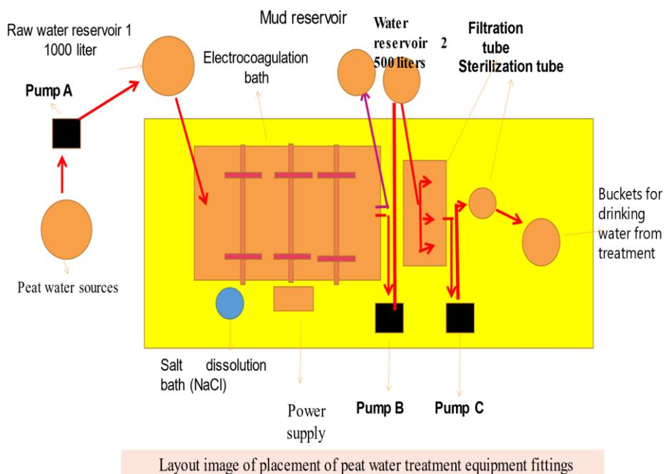
**Figure 2.** Layout Image of Placment of Peat Water Treatment Equipment Fitting
