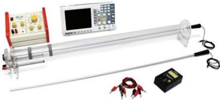
Gambar 5.10. Set Alat Praktikum Resonansi (Sumber: https://pudakscientific.com/image/set_907_tabung_resonansi.pdf )
